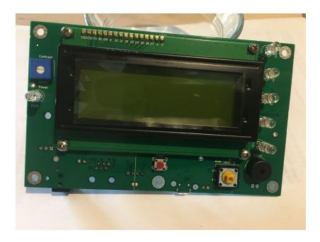
The GPAD device is designed to be used as a multi-purpose "alarm device". It has bright LEDs on the right that can be programmed to show "alarm level", and a built-in buzzer that can produce a variety of pitches. It has a "mute" button on the face and a large LCD display to show the cause of the panic condition.
