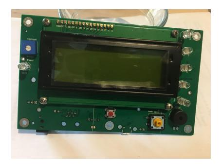
The GPAD device is designed to be used as a multi-purpose "alarm device." This device includes: bright LEDs on the right that can be programmed to show "alarm level," a built-in buzzer that can produce a variety of pitches, a "mute" button on its face, and a large LCD display to show the cause of the panic condition.
