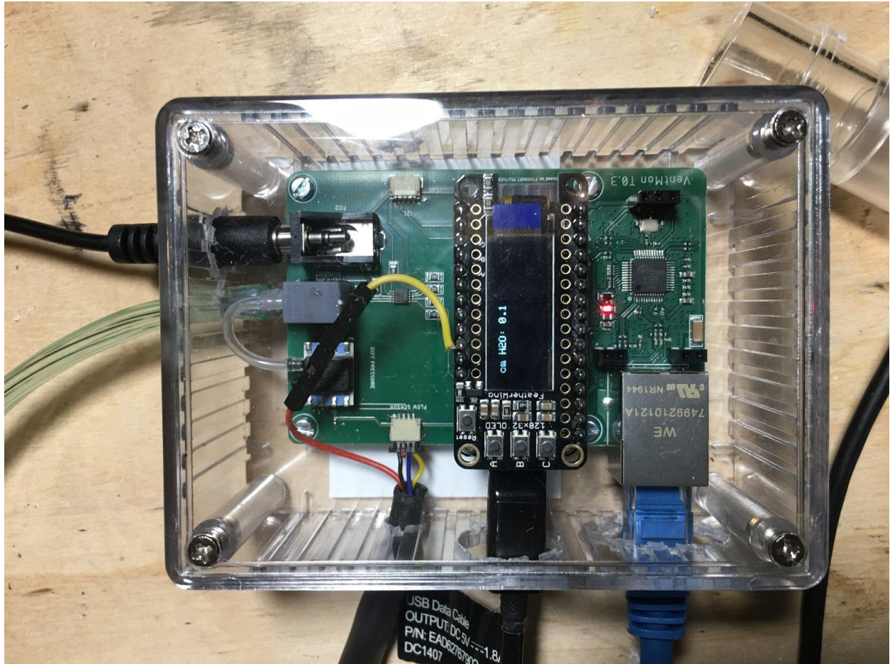
The VentMon T0.3 as assembled by Rob from the PCB designed by Lauria
